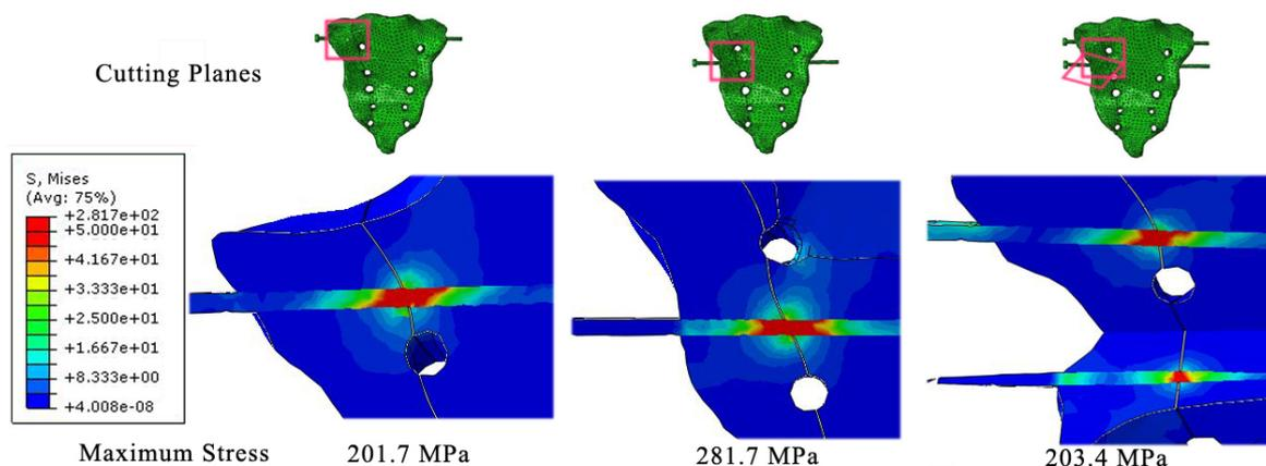
Figure 2. Contours of von Mises stress in cut views through the models with their maximum amounts
